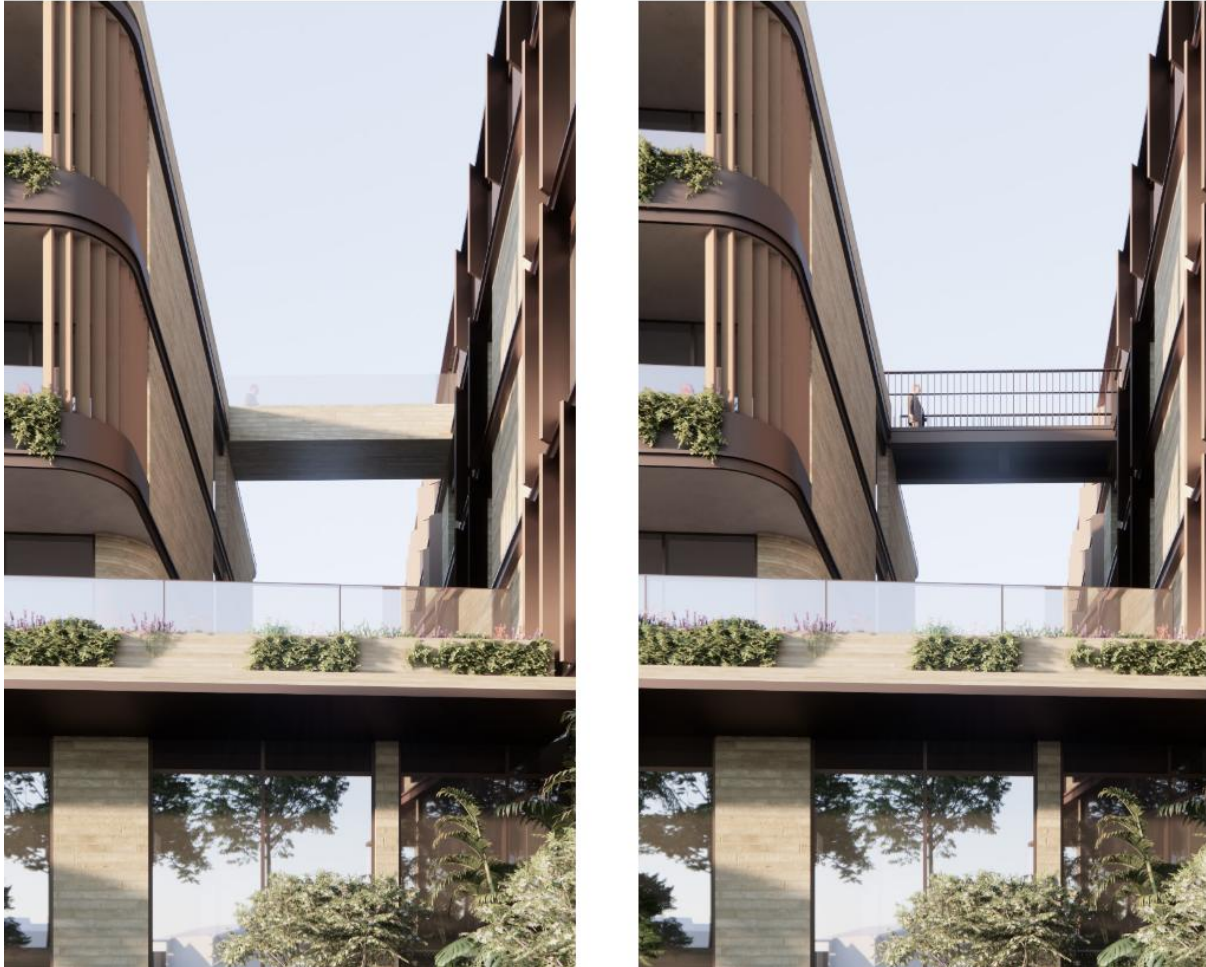
Figure 34: Proposed changes from the original concrete bridge/link between Buildings C1 and C2 to light weight metal palisade balustrading.
